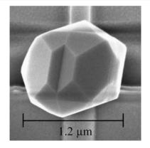
A method for the growth of single-crystal germanium on amorphous silicon by ultrahigh vacuum chemical vapor deposition at temperatures not exceeding 450 °C is presented. Growths proceed through constrictive channels and emerge with improved properties compared to as-deposited germanium. A description is given of the growth mechanism and its implications for design of the growth structure.
