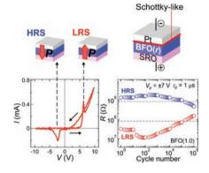
p-type Schottky-like Pt/BiFeO<sub>3</sub> interfaces show a bipolar-type resistive switching effect. A non-volatile resistive switching effect at Pt/BiFeO<sub>3</sub> interfaces induced by ferroelectric polarization reversal is reported. The devices show promising characteristics for use as non-volatile memories such as stable resistive switching without the need for any forming process, data retention of >10<sup>5</sup> s at room temperature, and endurance of >10<sup>5</sup> cycles.
