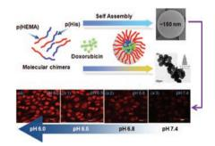
Uniform nanomicelles are fabricated via self-assembly of a series of biocompatible poly(2-hydroxyethyl methacrylate)-block-poly(L-histidine) hybrid materials. They are shown to be a suitable carrier for the pH-sensitive delivery of doxorubicin.
