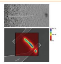
Scanning photocurrent spectroscopy is used to study the photovoltaic response of single heterostructure n-GaAs/InGaP/ p-GaAs core-multishell nanowire diodes. The proposed structure allows a selective wet etching of the individual shells and therefore a simple fabrication process. On the basis of a systematic characterization, good optoelectronic properties are demonstrated.
