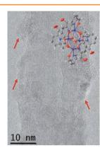
Two different routes that enable the electrostatic grafting of cationic single-molecule magnets (SMMs) onto the surface of chemically modified anionic multiwalled carbon nanotubes (MWNTs) are described. The chemical nature and physical properties of the resulting hybrids are discussed on the basis of the experimental techniques. The chemical nature of the SMM unit remains intact, while its magnetic response is significantly affected by the grafting process.
