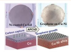
Homogenous growth of wafer-sized high-quality graphene is autonomously controlled by a novel substrate design in which a "smart" composite substrate with a self-evolving composition autonomously regulates the carbon content. The processing temperature spans from 1000 °C to 650 °C, the graphene layer number can be tuned from one to five, and the transparent conductive properties exceed the best reported for large-area graphenes.
