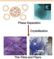
Taking inspiration from biomineralization, acidic additives are widely used to control calcium carbonate precipitation. It is shown that the positively charged additive poly(allylamine hydrochloride) (PAH) is also highly effective and it can direct the growth of thin films and fibers of CaCO3. These results are attributed to microphase separation of PAH in the presence of carbonate ions.
